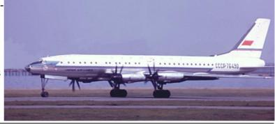
(rotate in opposite directions), essentially making it an eight-engined plane. (If you look carefully at an engine in the picture, you should notice two sets of propellers.)
