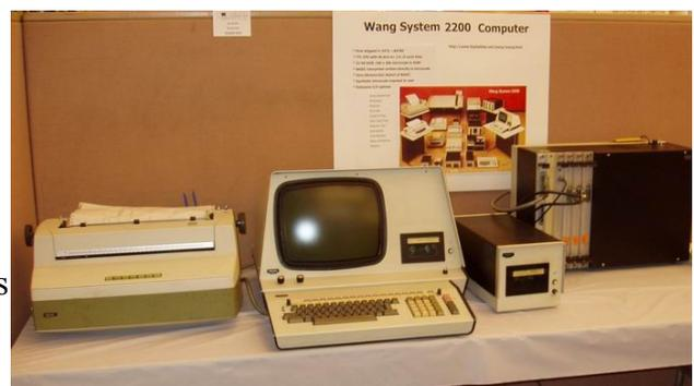
the computer. The printers in those days were of the 'daisy wheel' type (same as our IBM electric typewriter) so were not that fast and were limited to the characters on the daily wheel.
